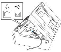
Carefully guide the USB cable into the trench as shown below, following the trench around and toward the back of the machine. Then, connect the cable to your Macintosh<sup>®</sup>.
