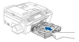
8 While holding the paper tray in place, pull out the paper support (1) until it clicks, and then unfold the paper support flap (2).
