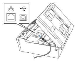
Carefully guide the USB cable into the trench as shown below, following the trench around and toward the back of the machine. Then, connect the cable to your Macintosh®.
