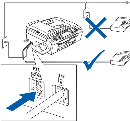
Set the receive mode to 'Manual' if you have an external answering machine. See the section 11 Choosing a Receive Mode on page 14. For more details, see Connecting an external TAD (telephone answering device) in Chapter 7 of the User's Guide.
