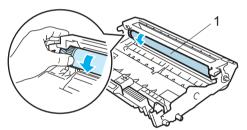
3 When you have found the mark on the drum that matches the print sample, wipe the surface of the OPC drum with a dry cotton swab until the dust or glue on the surface comes off.
