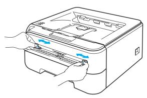
4 Using both hands, put one piece of paper or one transparency in the manual feed slot until the front edge of the paper or transparency touches the paper feed roller. When you feel the machine pull in the paper, let go.
