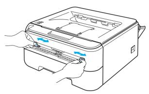
4 Using both hands, put one piece of paper or one envelope in the manual feed slot until the front edge of the paper or envelope touches the paper feed roller. When you feel the machine pull in the paper, let go.
