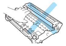
11 Put the toner cartridge back into the drum unit until you hear it lock into place. If you put the cartridge in properly, the green lock lever will lift automatically.
