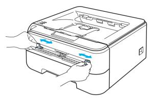
4 Using both hands put the paper in the manual feed slot with the side that is going to be printed on first facing up. Follow the instructions on the computer screen. Repeat this step until you have printed all the even-numbered pages.
