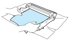
2 Turn the drum unit gear by hand while looking at the surface of the OPC drum (1).
