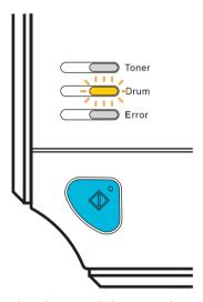
If the LED shows the message, it means the drum unit is near the end of its life. We recommend that you replace the drum unit with a new one before there is a noticeable deterioration in the print quality.
