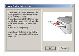
6 Remove the printed even-numbered pages from the output tray, and then put the first of the printed sheets back into the manual feed slot with the side to be printed on (the blank side) face up. Follow the instructions on the computer screen.
