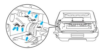
Push down the green lock lever and take the toner cartridge out of the drum unit.
