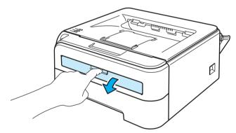
3 Using both hands, slide the manual feed slot paper guides to the width of the paper that you are going to use.
