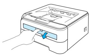
3 Using both hands, slide the manual feed slot paper guides to the width of the paper that you are going to use.
