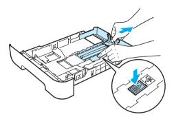
3 Put paper in the tray, and make sure that the paper is below the maximum paper mark (1). The side to be printed on must be face down.
