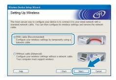
9 For configuration, you must temporarily connect your Brother wireless device (your printer) directly to a free port on your access point, hub or router using a network cable. When the following screen appears, insert the network cable to the access point and then to the printer. Click Next.
