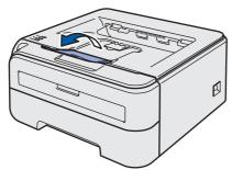
After the printer has finished warming up, the Ready LED / Go button (1) stops blinking and stays blue.
