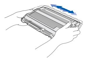
Put the drum unit and toner cartridge assembly into the machine.
