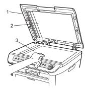
3 In the ADF unit, clean the white bar (1) and the scanner glass strip (2) underneath it with a soft lint-free cloth moistened with water.
