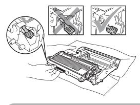
Make sure that you put in the toner cartridge correctly or it may separate from the drum unit.
