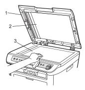
3 (DCP-7040 only) In the ADF unit, clean the white bar (1) and the scanner glass strip (2) underneath it with a soft lint-free cloth moistened with water.
