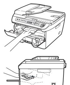
4 Put the drum unit and toner cartridge assembly back in the machine.
