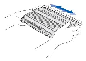
4. Put the drum unit and toner cartridge assembly into the machine.
