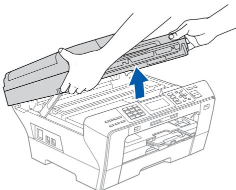
**b** Connect the USB cable to the USB socket marked with a
