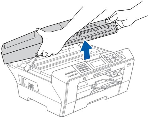
**b** Connect the USB cable to the USB socket marked with a
