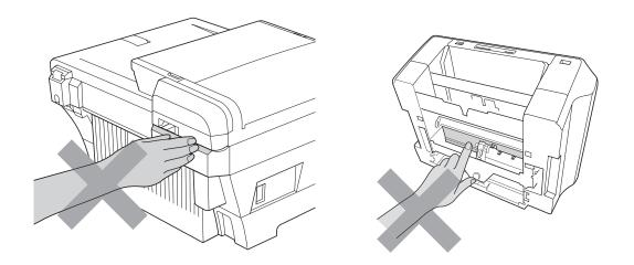
When moving the machine you must lift it from the base, by placing a hand at each side of the unit as shown in the illustration. DO NOT carry the machine by holding the scanner cover or the Outer Rear Cover.
