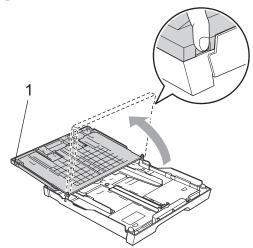
With both hands, gently press and slide the paper side guides (1) and then the paper length guide (2) to fit the paper size. Make sure that the triangular marks (3) on the paper side guides (1) and paper length guide (2) line up with the mark for the paper size you are using.
