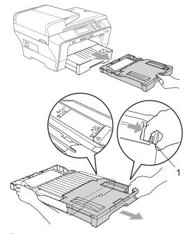
Open the paper tray cover and adjust the paper length guide (1) for the paper of Tray #1.
