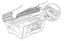
If ink gets on your skin or clothing immediately wash it off with soap or detergent. 8 Gently close the scanner cover using the finger holds on both sides of it as you push down on the Scanner Cover Support (1).
