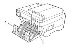
Clean the Paper Pick-up Roller (1) with isopropyl alcohol on a cotton swab.
