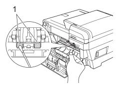
Close the Inner Rear Cover back and the Outer Rear Cover. Make sure the cover is closed correctly.
