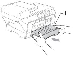
Pull out the jammed paper (1) and press Stop/Exit.
