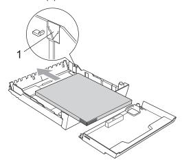
6 Gently adjust the paper side guides with both hands to fit the paper stack. Make sure the paper side guides touch the sides of the paper.
