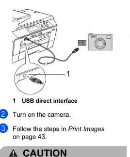
To prevent damage to your machine, do not connect any device other than a digital camera or USB Flash memory drive to the USB direct interface.
