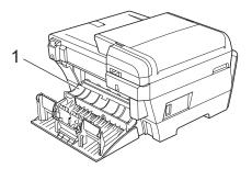
6 Close the Outer Rear Cover. Make sure the cover is closed correctly.
