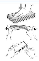
2 Put envelopes or post cards in the paper tray with the address side down and the leading edge (top of the envelopes) in first. With both hands, gently press and slide the paper side guides (1) and paper length guide (2) to fit the size of the envelopes or post cards.
