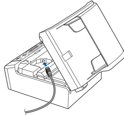
**c** Carefully guide the USB cable through the trench as shown below, following the trench around and toward the back of the machine. Then connect the cable to your Macintosh®.
