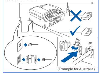
Set the receive mode to External TAD if you have an external answering machine. See Choose a Receive Mode on page 8. For additional details, see Connecting an external TAD (telephone answering device) in Chapter 7 of the User's Guide.
