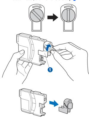
Take care to match the colour of the lever 1 with the cartridge colour 2, as shown in the diagram below.
