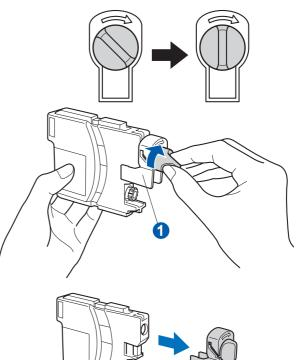
Take care to match the colour of the lever 1 with the cartridge colour 2, as shown in the diagram below.
