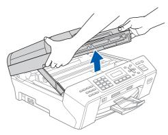
b Connect the network cable to the LAN socket marked with a R symbol. You will find the LAN socket inside the machine on the left as shown below.
