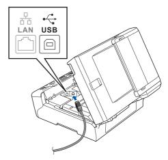
Carefully guide the USB cable through the trench as shown below, following the trench around and toward the back of the machine. Then connect the cable to your Macintosh®.
