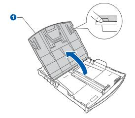
C With both hands, gently press and slide the paper side guides 1 and then the paper length guide 2 to fit the paper size.
