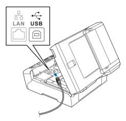
Carefully guide the USB cable through the trench as shown below, following the trench around and toward the back of the machine. Then connect the cable to your Macintosh<sup>®</sup>.
