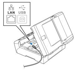
C Carefully guide the network cable to the trench as shown below, following the trench around and toward the back of the machine. Then, connect the cable to your network.
