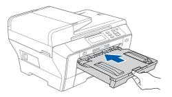
While holding the paper tray in place, pull out the paper support **1** until it clicks, and then unfold the paper support flap **2**.
