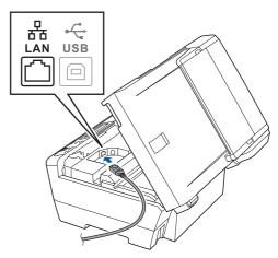
Carefully guide the network cable to the trench as shown below, following the trench around and toward the back of the machine. Then, connect the cable to your network.
