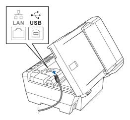
Carefully guide the USB cable through the trench as shown below, following the trench around and toward the back of the machine. Then connect the cable to your Macintosh<sup>®</sup>.
