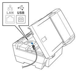
C Carefully guide the USB cable through the trench as shown below, following the trench around and toward the back of the machine. Then connect the cable to your computer.
