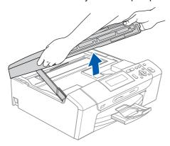
Connect the USB cable to the USB socket marked with a symbol. You will find the USB socket inside the machine on the right as shown below.
