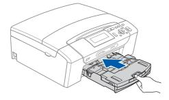
While holding the paper tray in place, pull out the paper support 1 until it clicks, and then unfold the paper support flap 2.
