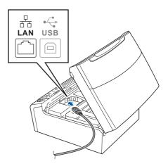
Carefully guide the network cable to the trench as shown below, following the trench around and toward the back of the machine. Then, connect the cable to your network.
