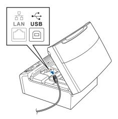
Carefully guide the USB cable through the trench as shown below, following the trench around and toward the back of the machine. Then connect the cable to your Macintosh<sup>®</sup>.
