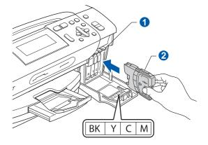
Install each ink cartridge in the direction of the arrow on the label.
