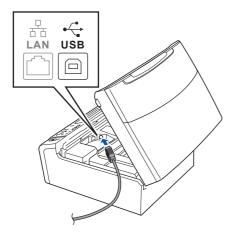
Carefully guide the USB cable through the trench as shown below, following the trench around and toward the back of the machine. Then connect the cable to your computer.
