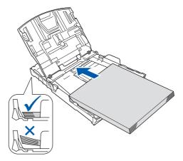
Gently adjust the paper side guides to the paper with both hands. Make sure that the paper side guides touch the edges of the paper.
