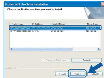
If your machine shows **APIPA** in the **IP Address** field, click **Configure IP Address** and enter an IP address for your machine that is suitable for your network.
