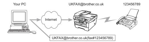
You can also send E-mail from your computer and have it relayed to a conventional fax machine. The method of entering the phone number of the conventional fax machine that will receive the relayed E-mail will vary depending on the mail application you are using. The following are some examples of different mail applications:
