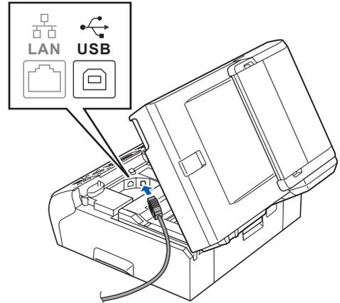
**c** Carefully route the USB cable through the trench and out the back of the machine as shown below and connect the cable to your Macintosh®.
