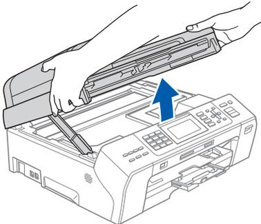
**b** Connect the USB cable to the USB socket marked with a
