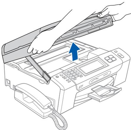
**b** Connect the USB cable to the USB socket marked with a
