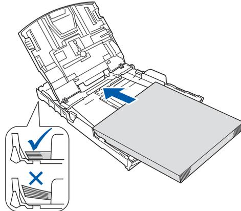
**f** Gently adjust the paper side guides to the paper with both hands. Make sure that the paper side guides touch the edges of the paper.
