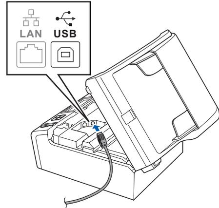
**c** Carefully guide the USB cable through the trench as shown below, following the trench around and toward the back of the machine. Then connect the cable to your Macintosh®.
