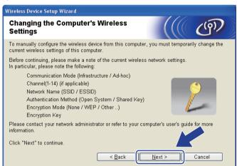
To communicate with the un-configured wireless machine, temporarily change the wireless settings on your computer to match the machine's default settings shown on this screen. Check the box after you confirm these settings, and then click **Next**.
