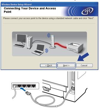
11 Choose the machine you wish to configure, and click **Next**. If the list is blank, check if the access point and the machine are powered on, and then click **Refresh**.
