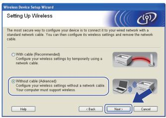
Read the **Important Notice** to enable the wireless interface. Hold down the **Go** button for 10 seconds, and then release the **Go** button when the printer prints a Network Configuration page. Check the box after you confirm the wireless setting is enabled, and then click **Next**.
