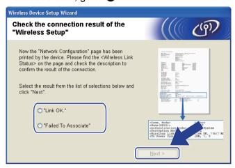
Click **Finish**. Wireless setup was unable to associate with a wireless network. This is probably due to incorrect security settings. Reset the print server back to its factory default settings (see *Reset the network settings to the factory default* on page 118). Confirm the security settings of your wireless network and try starting from **6** again.
