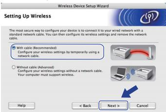
Connect the Brother wireless device to your access point using a network cable and click Next.
