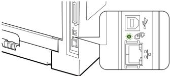
■ The LED is on: Your machine is connected to the wireless network.
