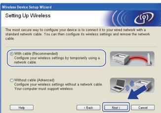
10 Connect the Brother wireless device to your access point using a network cable and click Next.
