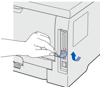
**i** When this screen appears, make sure the printer power switch is on. Connect the USB cable to the USB connector marked with a
