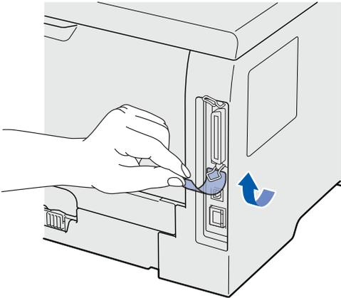
**b** Connect the USB cable to the USB connector marked with a
