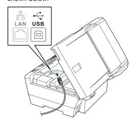
Carefully guide the USB cable through the trench as shown below, following the trench around and toward the back of the machine. Then connect the cable to your computer.
