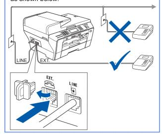
Set the receive mode to External TAD if you have an external answering machine. See Choose a Receive Mode on page 8. For additional details, see Connecting an external TAD (telephone answering device) in Chapter 7 of the User's Guide.
