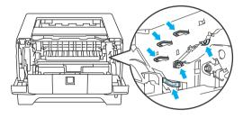
Clean the primary corona wire inside the drum unit by gently sliding the blue tab from right to left and left to right several times.
