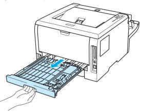
9 Pull the jammed paper out of the printer or the duplex tray.
