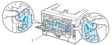
5 Using both hands, gently pull the jammed paper out of the fuser unit.
