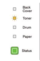
If the LED shows this message, the toner cartridge is near the end of its life. Buy a new toner cartridge and have it ready before you get a Replace Toner message. To replace the toner cartridge, see *Replacing the toner cartridge* on page 95.
