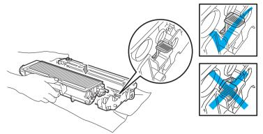
8 Open the front cover. Put the drum unit and toner cartridge assembly back in the printer.
