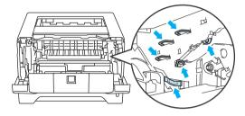
B Push down the blue lock lever and take the toner cartridge out of the drum unit.
