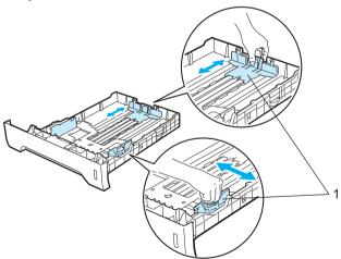
3 Put paper in the tray, and make sure that the paper is below the maximum paper mark (▼▼▼). The side to be printed on must be face down.
