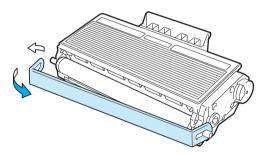
6 Put the new toner cartridge firmly into the drum unit until you hear it lock into place. If you put it in properly, the lock lever will lift automatically.
