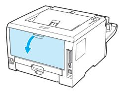
Pull the tabs at the left and right hand sides toward you to open the fuser cover (1). 4
