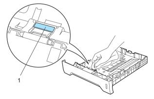
5 Wipe the two paper pick-up rollers (1) inside the printer.
