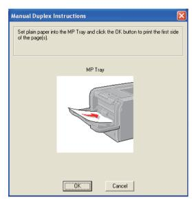
5 Remove the printed even-numbered pages from the output tray and then, in the same order <sup>1</sup>, put them back into the MP tray. Put the paper with the side to be printed on (the blank side) face up. Follow the instructions on the computer screen.
