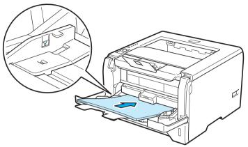
5 While pressing the paper-guide release lever (1), slide the paper guide to fit the paper size.
