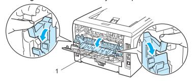
5 Using both hands, gently pull the jammed paper out of the fuser unit.
