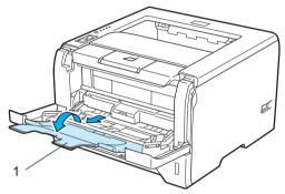
3 Lift up the support flap to prevent paper from sliding off the face-down output tray, or remove each page as soon as it comes out of the printer.
