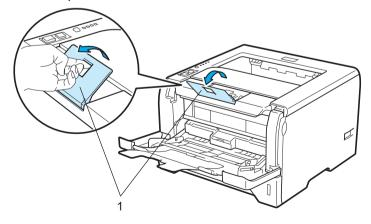
4 Put paper in the MP tray. Make sure that the paper stays under the maximum paper mark (▼) on both sides of the tray. The side to be printed on must be face up with the leading edge (top of the paper) in first.
