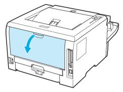
4 Pull the tabs at the left and right hand sides toward you to open the fuser cover (1).
