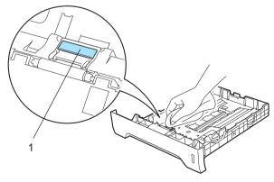
5 Wipe the two paper pick-up rollers (1) inside the printer.
