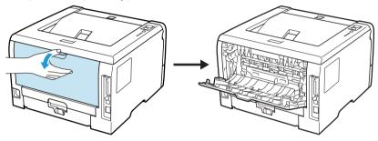
2 <For printing envelopes only> Pull down the two gray levers, one on the left-hand side and one on the right-hand side, toward you as shown in the illustration below.
