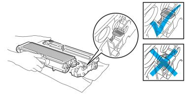
8 Open the front cover. Put the drum unit and toner cartridge assembly back in the printer.
