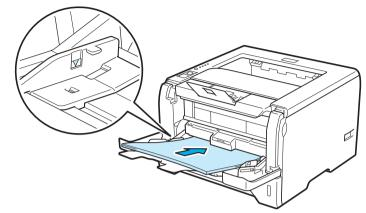
6 While pressing the paper-guide release lever (1), slide the paper guide to fit the paper size.
