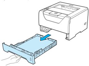
5 Pull the jammed paper down and out of the printer.
