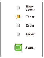
If the LED shows this message, the toner cartridge is near the end of its life. Buy a new toner cartridge and have it ready before you get a Replace Toner message. To replace the toner cartridge, see *Replacing the toner cartridge* on page 95.
