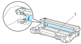
3) When you have found the mark on the drum that matches the print sample, wipe the surface of the OPC drum with a dry cotton swab until the dust or glue on the surface comes off.
