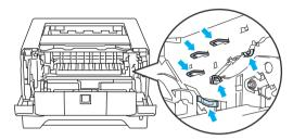
3 Clean the primary corona wire inside the drum unit by gently sliding the blue tab from right to left and left to right several times.
