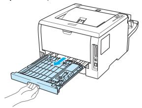
9 Pull the jammed paper out of the printer or the duplex tray.
