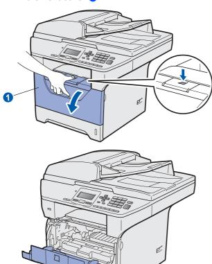
C Unpack the drum unit and toner cartridge assembly.
