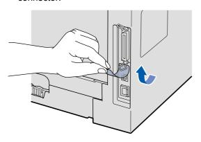
Connect the USB cable to the USB connector on the machine marked with the symbol. Then connect the cable to your computer.
