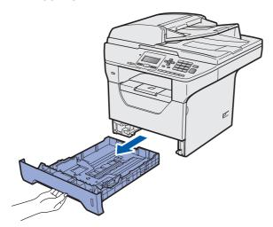
While pressing the blue paper-guide release lever 1, slide the paper guides to fit the paper size you are loading in the tray. Make sure that the guides are firmly in the slots.
