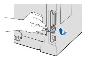
Onnect the USB cable to the USB connector on the machine marked with the symbol. Then connect the cable to your computer.
