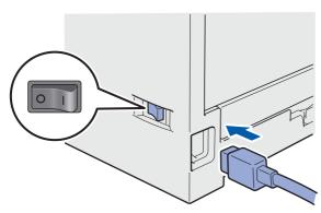
Plug the AC power cord into an AC outlet. Turn the power switch on.
