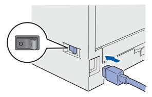
b Plug the AC power cord into an AC outlet. Turn the power switch on.
