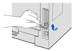
Connect the USB cable to the USB connector on the machine marked with the espective symbol. Then connect the cable to your computer.
