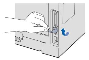
Connect the USB cable to the USB connector on the machine marked with the 😪 symbol. Then connect the cable to your computer.
