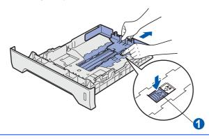
**C** Fan the stack of paper well to avoid paper jams and misfeeds.
