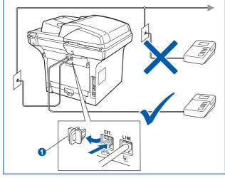
Set the receive mode to External TAD if you have an external answering machine. See Choose the correct Receive Mode on page 7. For additional details, see Connecting an external TAD (telephone answering device) in Chapter 7 of the User's Guide.
