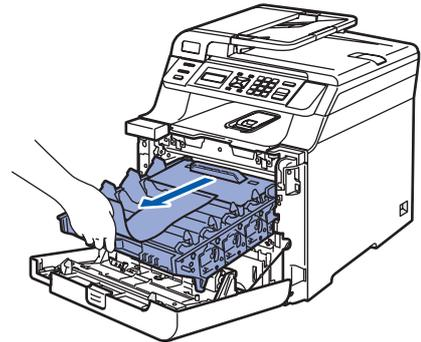
**5** Remove the orange packing material as shown in the illustration below.
