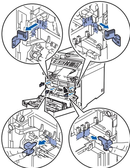
**4** Hold the green handle of the drum unit. Lift the drum unit up and then pull it out until it stops.
