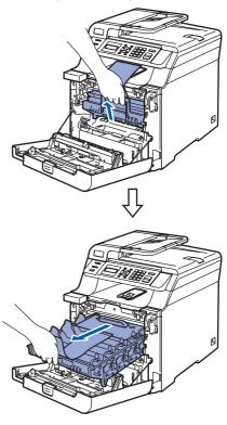
Remove the orange packing material as shown in the illustration below.
