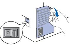
2 Connect the AC power cord to the machine.
