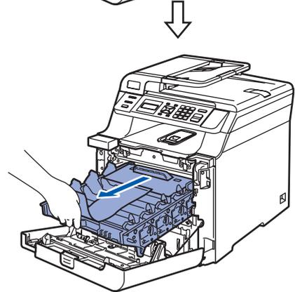
5 Remove the orange packing material as shown in the illustration below.
