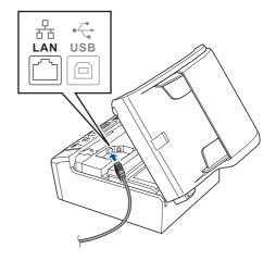
Carefully guide the network cable through the trench as shown below, following the trench around and toward the back of the machine. Then, connect the cable to your network.
