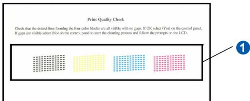
**c** If all lines are clear and visible, press **1** (Yes) on the dial pad to finish the quality check and go to step **6**.
