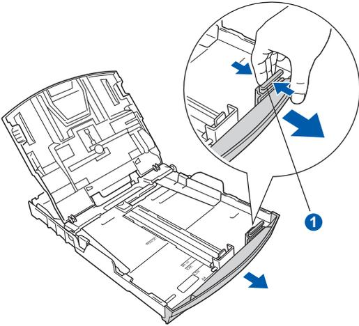
**f** Gently adjust the paper side guides to the paper with both hands. Make sure that the paper side guides touch the edges of the paper.
