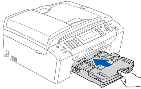
**i** While holding the paper tray in place, pull out the paper support ① until it clicks, and then unfold the paper support flap ②.
