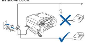
Set the receive mode to Manual if you have an external answering machine. See Choose a Receive Mode on page 7. For additional details, see Connecting an external TAD (telephone answering device) in Chapter 7 of the User's Guide.
