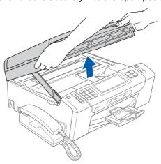
b Connect the network cable to the LAN socket marked with a R symbol. You will find the LAN socket inside the machine on the left as shown below.
