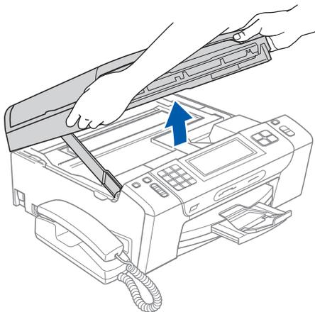
**b** Connect the USB cable to the USB socket marked with a
