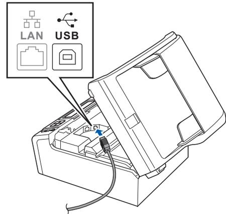
**c** Carefully route the USB cable through the trench and out the back of the machine as shown below and connect the cable to your Macintosh.
