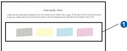
**c** If all lines are clear and visible, press **Yes** to finish the quality check and go to step **7**.
