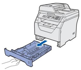
While pressing the blue paper-guide release lever 1, slide the paper guides to fit the paper size you are loading in the tray. Make sure that the guides are firmly in the slots.
