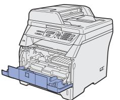
C Unpack the drum unit and toner cartridge assembly.
