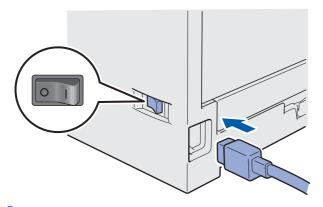
Plug the AC power cord into an AC outlet. Turn the power switch on.
