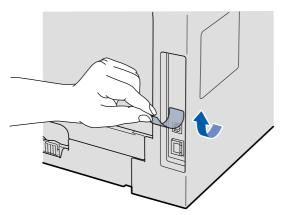
Connect the USB cable to the USB connector on the machine marked with the 😪 symbol. Then connect the cable to your computer.
