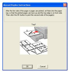
When printing to the Back output tray put the paper back in the tray in the opposite order it came out.
