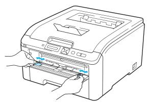
4 Using both hands put the paper in the manual feed slot with the side that is going to be printed on first facing up. Send the data to the printer, then follow the instructions on the computer screen. Repeat this step until you have printed all the even-numbered pages.
