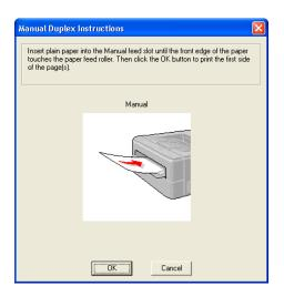
Remove the printed even-numbered pages from the output tray and then, in the same order <sup>1</sup>, put them back into the manual feed slot. Put the paper with the side to be printed on (the blank side) face up. Follow the instructions on the computer screen.
