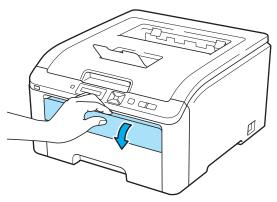
2 Using both hands, slide the manual feed slot paper guides to the width of the paper that you are going to use.
