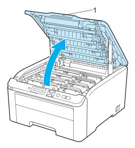
2 See the print sample to identify the color causing the problem. The color of the spots is the color of the drum you should clean. For example, if the spots are cyan, you should clean the drum for cyan. Take out the drum unit and toner cartridge assembly of the color causing the problem.
