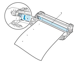
6 When you have found the mark on the drum that matches the print sample, wipe the surface of the OPC drum with a dry cotton swab until the dust or glue on the surface comes off.
