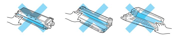
3 Hold the green handle of the belt unit and lift the belt unit up, then pull it out.
