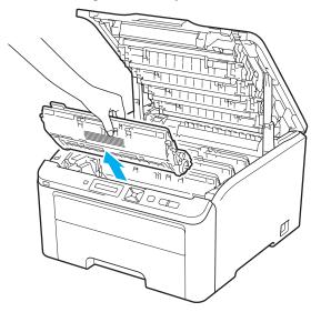
3 Push down the green-labeled lock lever (1) and take the toner cartridge out of the drum unit.
