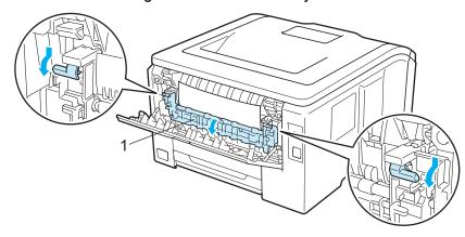
4 Using both hands, gently pull the jammed paper out of the fuser unit.
