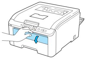
3 <For printing envelopes only> Pull down the two grey levers, one on the left-hand side and one on the right-hand side, toward you as shown in the illustration below.
