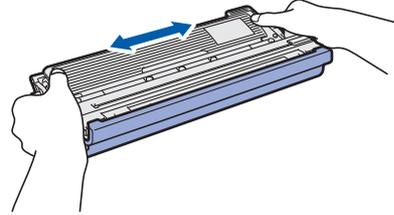
**b** Remove the protective cover by pulling on the tab as shown in the illustration.
