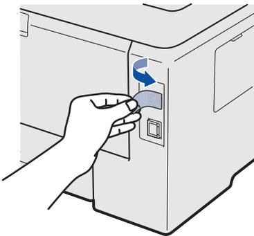
**i** When this screen appears, turn on the printer's power switch. Connect the USB cable to the USB connector marked with the
