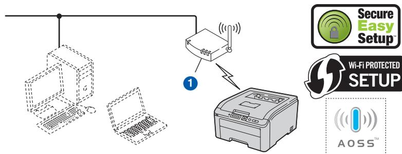
If your wireless access point 1 supports either SecureEasySetup™, Wi-Fi Protected Setup (PBC<sup>1</sup>) or AOSS™, you do not need to use a computer to configure the wireless settings. The access point/router and your printer can automatically negotiate using the SecureEasySetup™, Wi-Fi Protected Setup or AOSS™ procedure.
