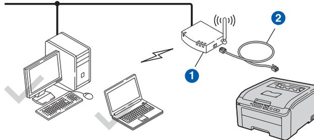
If there is an Ethernet Hub or Router in the same network as the wireless access point 1 of your printer, you can temporarily connect the Hub or Router to the printer using an Ethernet cable 2, this is an easy way to configure the printer. You can then remotely configure the printer from a computer on the network.
