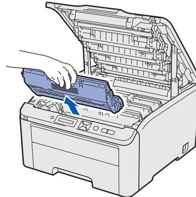
Attach the protective cover to each of the drum unit and toner cartridge assemblies.
