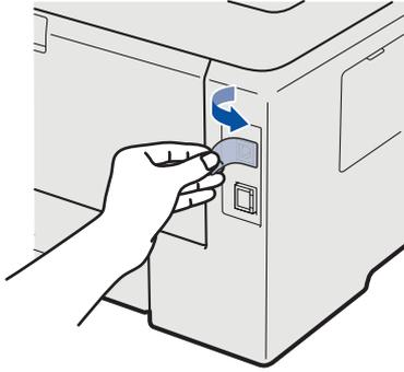
**b** Connect the USB cable to the USB connector marked with a
