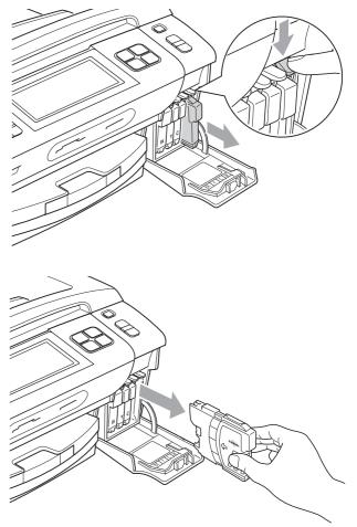
Open the new ink cartridge bag for the colour shown on the LCD, and then take out the ink cartridge.
