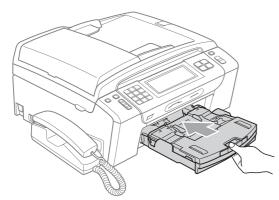
9 While holding the paper tray in place, pull out the paper support (①) until it clicks, and then unfold the paper support flap (②).
