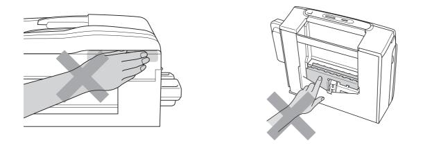
When moving the machine you must lift it from the base, by placing a hand at each side of the unit as shown in the illustration. DO NOT carry the machine by holding the scanner cover or Jam Clear Cover.
