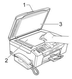
In the ADF unit, clean the white bar (1) and the glass strip (2) with a lint-free cloth moistened with a non-flammable glass cleaner.
