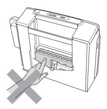
When moving the machine you must lift it from the base, by placing a hand at each side of the unit as shown in the illustration. DO NOT carry the machine by holding the scanner cover or Jam Clear Cover.
