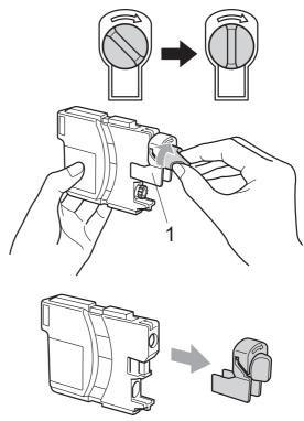
5 Each colour has its own correct position. Insert the ink cartridge in the direction of the arrow on the label.
