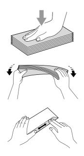
Put envelopes or postcards into the paper tray with the side to be printed on face down, and the shortest edge in first as shown in the illustration. We recommend you load one extra envelope or postcard. With both hands, gently press and slide the paper side guides (1) and paper length guide (2) to fit the size of the envelopes or postcards.
